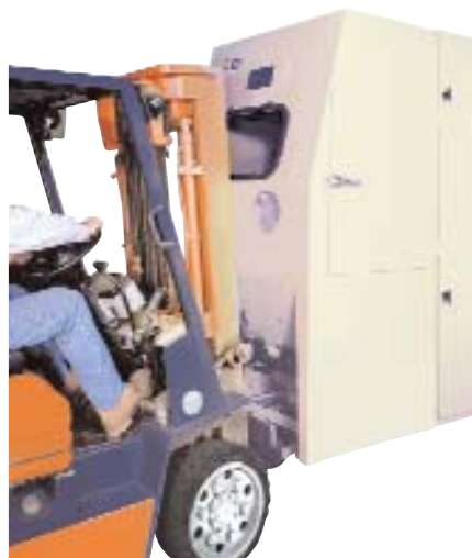
Figure 1: Industrial air-blast cabinets are available in a variety of standard configurations, including compact, easily transportable units that integrate blasting, media-reclamation, and dust-collection hardware within a single enclosure (left) and ergonomic models that improve operator efficiency over extended work periods (right).
