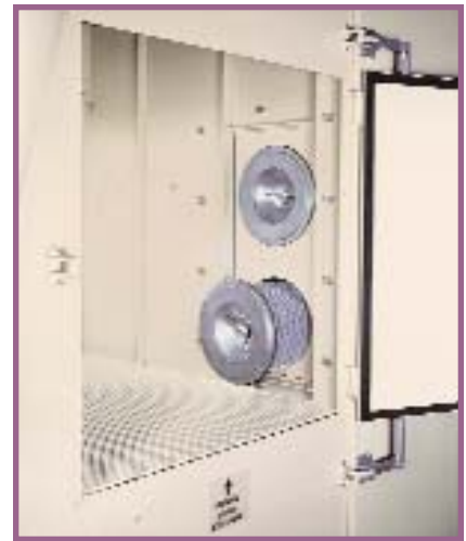
Figure 4: For dust collection, cartridge filters have grown in popularity because of long life, ease of replacement, and high efficiency.
